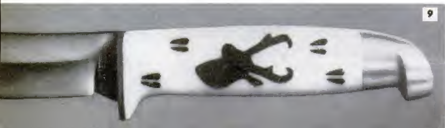
Roughly shaped handle is given a secondary sanding with 180-grit paper and then a final sanding with 320-grit paper, as above, both sandpapers being used wet. After sanding has resulted in desired shape, handle is given final polishing with cloth
